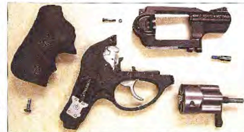
The LCR, stripped down and ready for maintenance and cleaning.
